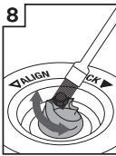
8 Clean lower burr with cleaning brush
